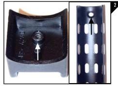
To install the rear ghost ring sight begin by placing the guide post of the large ghost ring sight into the pilot hole at the rear of the heatshield as seen in Figure 2.
