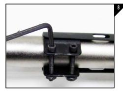
Install the provided (2) screws and nuts and tighten securely as seen in Figure 8.
