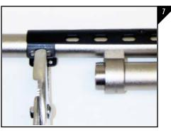
Tighten the front clamp around the barrel as seen in Figure 7.
